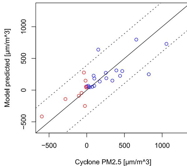
Figure 33 Comparison of PM2.5 measured by cyclone samplers and the prediction using PM10 measurements and duration of impactor samplers. The solid line denotes  $X=Y$ , and the dashed lines denote the 95%-CI of the model-fit residuals. Cyclone measurements of positive values were presented by blue dots, and negative values were by red dots.
