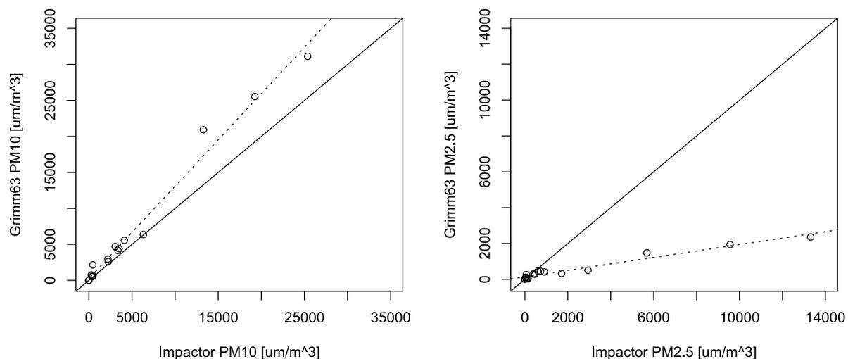
Figure 14 Comparisons between Grimm 63 and impactor samplers on PM10 (left) and PM2.5 (right) measurements. The solid lines denote  $x=y$ . The dashed lines denote the regression lines (unit  $\mu\text{m}/\text{m}^3$ ):  $Gri63_{pm10} = 251.7 + 1.29 \times \text{Impactor}$  and  $Gri63_{pm2.5} = 140.4 + 0.18 \times \text{Impactor}$ .
