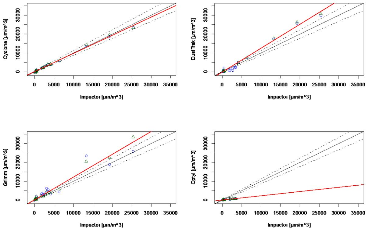
Figure 21 Comparisons between the impactor sampler measurements and four alternative methods on PM10. The blue circles and green triangles represent the measurement from one of the two units, respectively. The red solid line denote the orthogonal regression line. The black solid line denotes x=y regression line, and the dashed lines denote the interval of the desirable accuracy.
