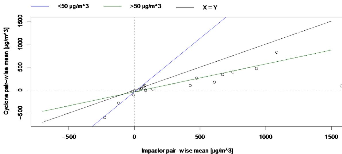
Figure 10 Comparison of the pair-wise mean between the impactor samplers and cyclone samplers on PM<sub>2.5</sub>. Blue (<50  $\mu\text{g}/\text{m}^3$ ) and green solid ( $\geq 50 \mu\text{g}/\text{m}^3$ ) lines demonstrate the linear regression lines at two concentration ranges with respect to the apparent concentrations measured by the impactor samplers. The black solid line denotes  $x = y$ .
