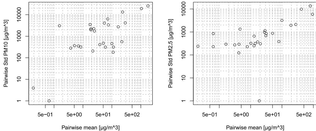
Figure 2 The pairwise mean and standard deviation of the impactor sampler measurements on PM10 (left) and PM2.5 (right). The pairwise mean on both plots were corrected for the offset to avoid negative values.
