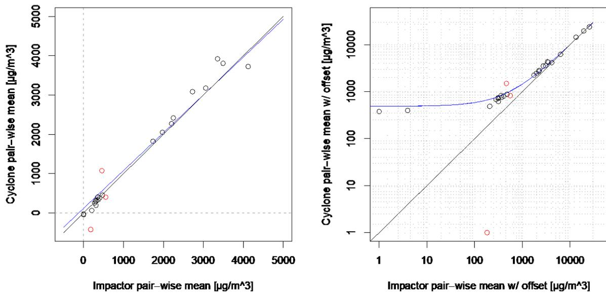
Figure 8 Comparison of the pair-wise mean between the impactor samplers and cyclone samplers on PM10 plotted in linear (left) and log-scale (right, with the offset shifted so that all values were  $\geq 1$ ). Blue solid line denotes the linear regression line (excluding outliers which are marked in red), and the black solid line denotes  $x = y$ .
