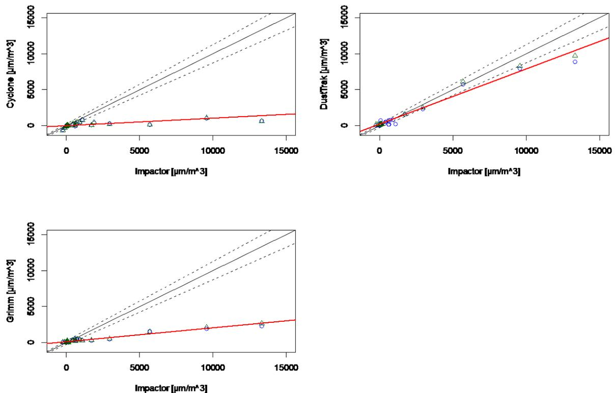
Figure 12 Comparisons between the impactor sampler measurements and four alternative methods on PM<sub>2.5</sub>. The blue circles and green triangles represent the measurement from one of the two units, respectively. The red solid line denote the orthogonal regression line. The black solid line denotes  $x=y$  regression line, and the dashed lines denote the interval of the desirable accuracy.
