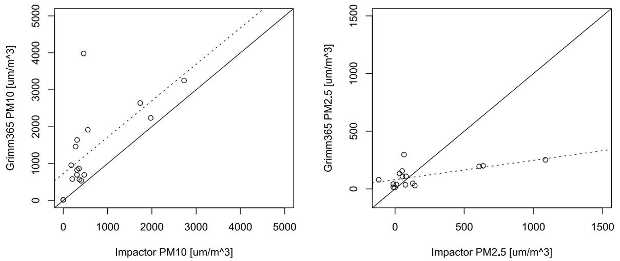
Figure 15 Comparisons between Grimm 365 and impactor samplers on PM10 (left) and PM2.5 (right) measurements. The solid lines denote  $x=y$ . The dashed lines denote the regression lines (unit  $\mu\text{m}/\text{m}^3$ ):  $Gri365_{pm10} = 728.1 + 0.99 \times \text{Impactor}$  and  $Gri365_{pm2.5} = 80.3 + 0.17 \times \text{Impactor}$ .
