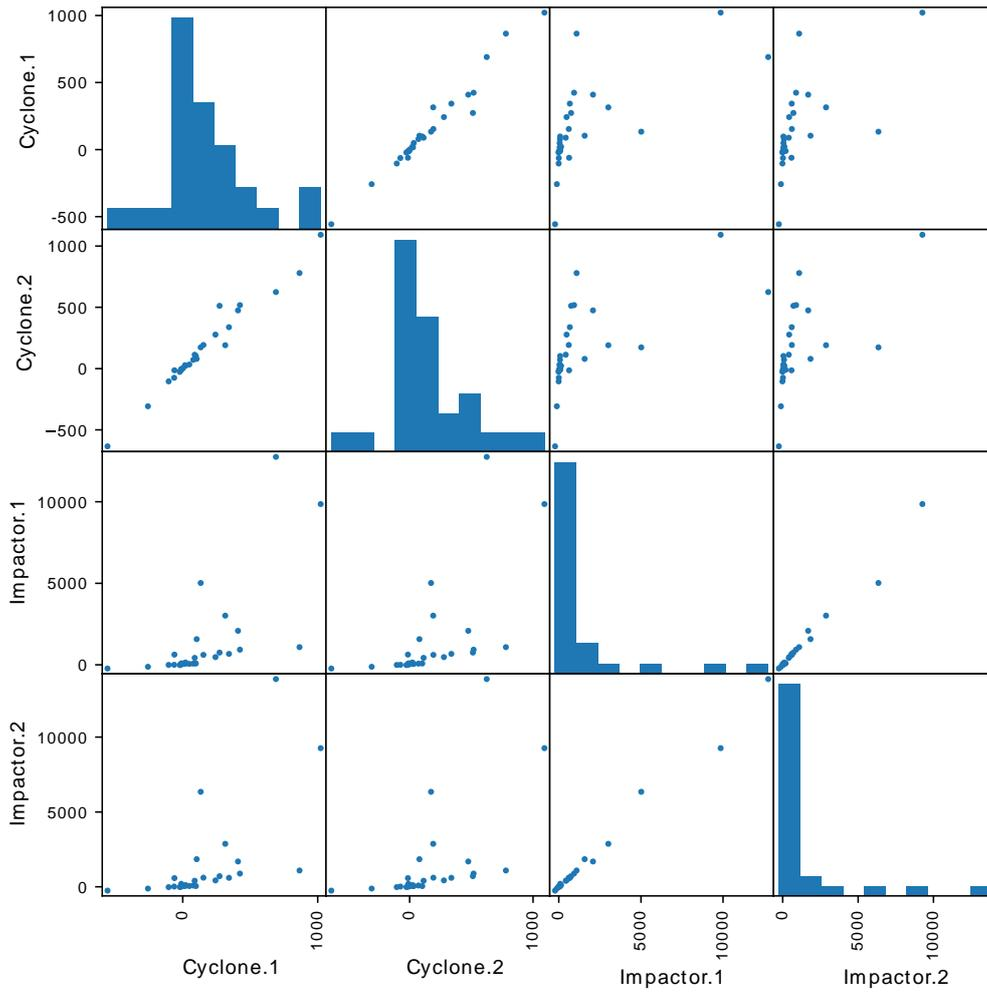
Figure 9 Scatter plots of the cyclone and impactor sampler measurement results on PM<sub>2.5</sub> (unit =  $\mu\text{g}/\text{m}^3$ ). The number after the device name denotes the ID of the measuring unit. The presented dataset contains 27 measurement trials.
