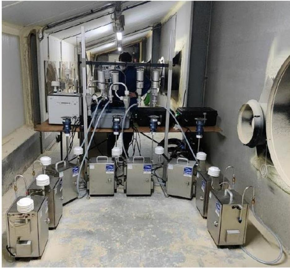
Figure 1: Set-up for simultaneous measurement with the different devices for measuring PM10 and PM2.5 concentrations in poultry houses.
