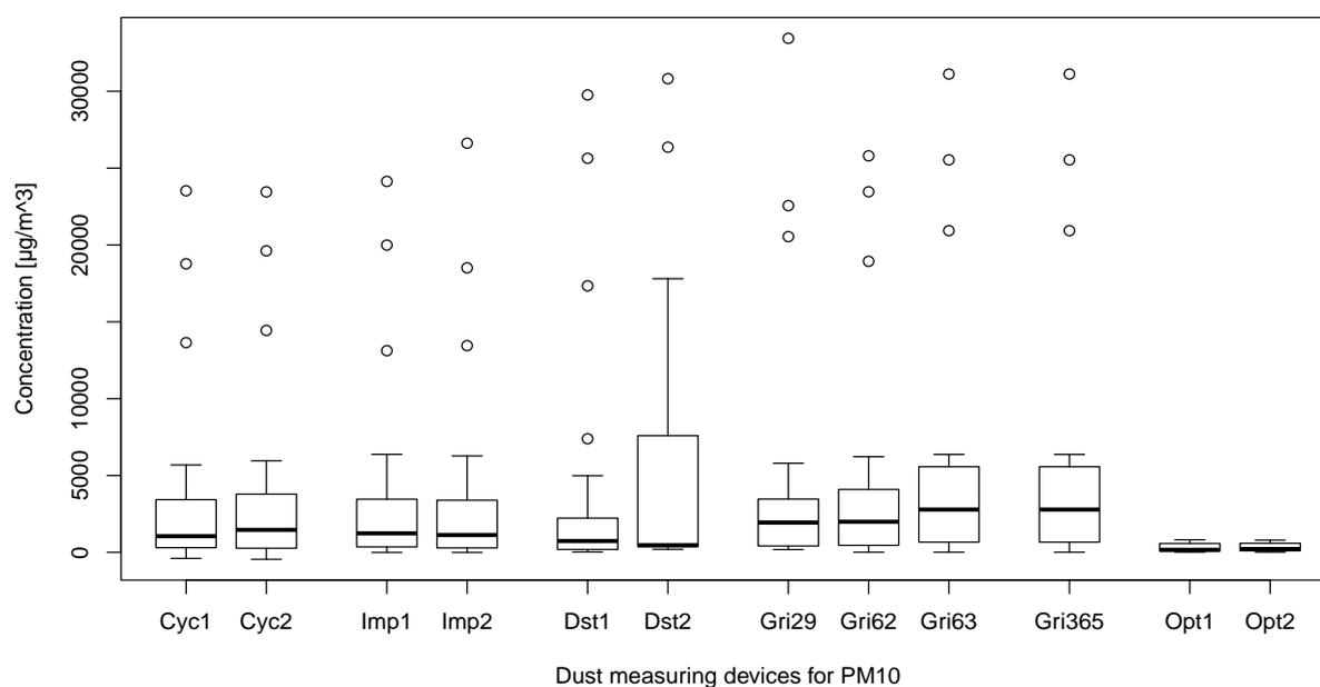
Figure 4 Summary of the measured PM10 concentrations by the dust measuring devices: Cyc – cyclone, Imp – impactor, Dst – DustTrak, Gri – Grimm, Opt – Optyl. The circles denotes outliers which are determined based on the 1.5×IQR rule.
