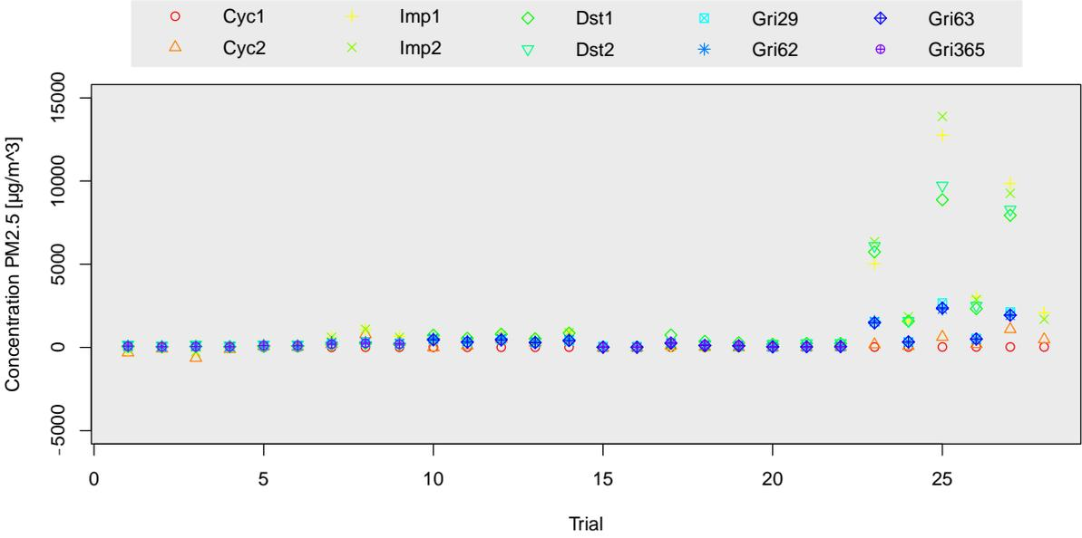
Figure 5 The measured PM2.5 concentrations in each trial by the dust measuring devices: Cyc – cyclone, Imp – impactor, Dst – DustTrak, Gri – Grimm, Opt – Optyl.
