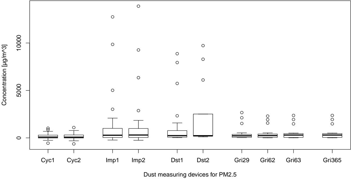
Figure 6 Summary of the measured PM2.5 concentrations by the dust measuring devices: Cyc – cyclone, Imp – impactor, Dst – DustTrak, Gri – Grimm. The circles denotes outliers which are determined based on the 1.5×IQR rule.
