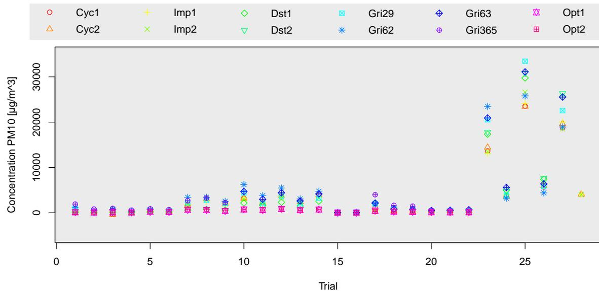
Figure 1 The measured PM10 concentrations in each trial by the dust measuring devices: Cyc – cyclone, Imp – impactor, Dst – DustTrak, Gri – Grimm, Opt – Optyl.
