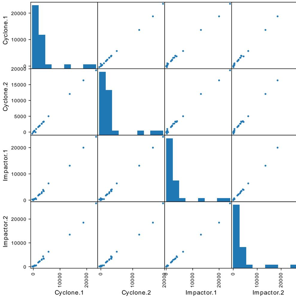
Figure 7 Scatter plots of the cyclone and impactor sampler measurement results on PM10 (unit =  $\mu\text{g}/\text{m}^3$ ). The number after the device name denotes the ID of the measuring unit. The presented dataset contains 27 measurement trials.
