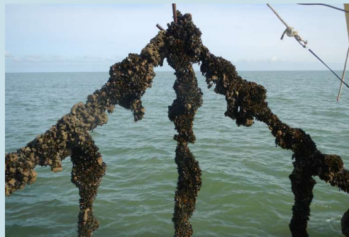
Biobased ropes deployed as mussel droppers at sea being tested on biodegradability. (©ILVO)
