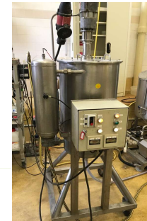
2 step extraction process Total volume = 74 L
