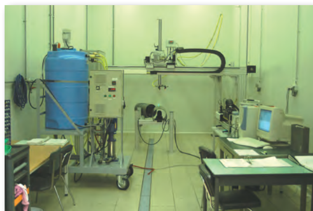
PDPA laser based measuring set-up of for measuring droplet size and velocity measurements of spray nozzles
