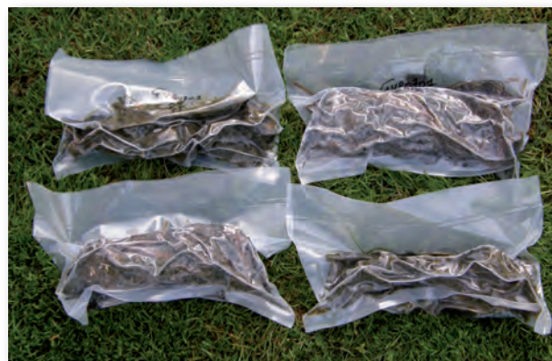
Labscale silages made by vacuum packing the forages in polyethylene bags
