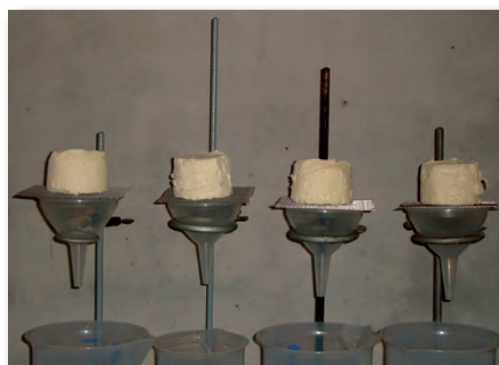
Start of melting behaviour of ice cream with modified milk fatty acid composition
