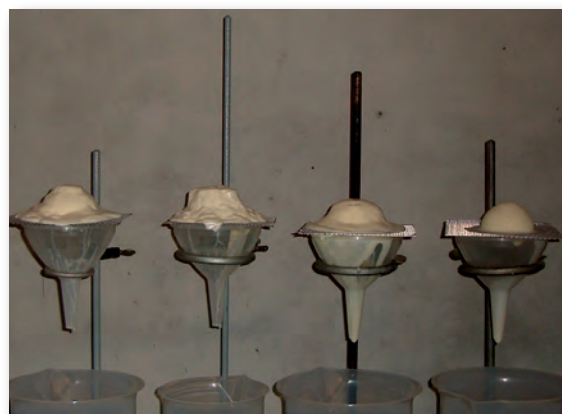
End of melting behaviour of ice cream with modified milk fatty acid composition
