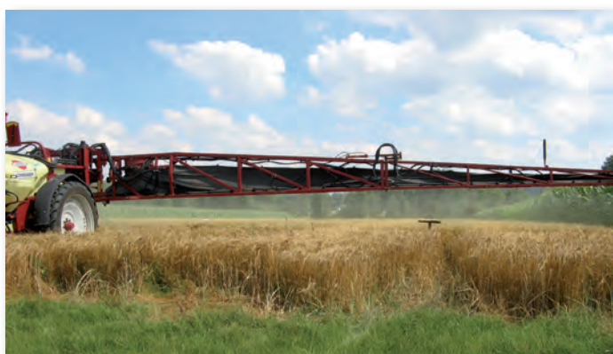
Field measurement to investigate the effect of crop type on the amount of spray drift
