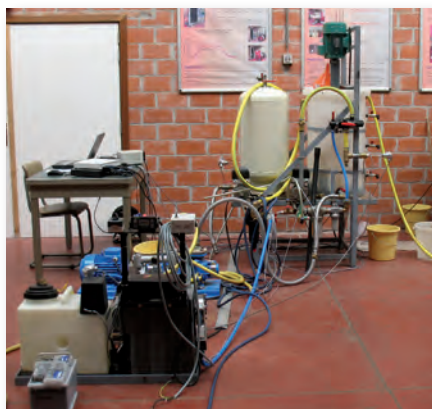
The modular spray application system
