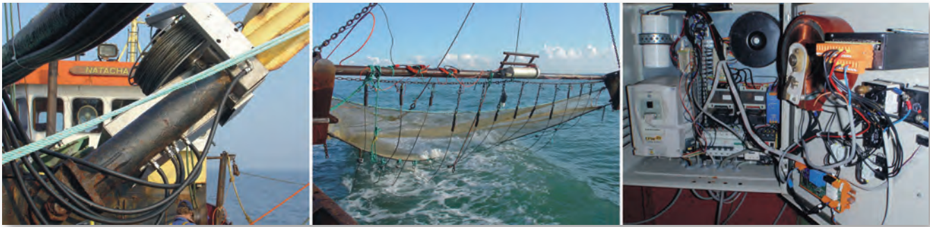
Figure 7: Installed equipment on board of the testing vessel. From left to right: electrical cable winch; pulse trawl with mounted impulse generator; control box
