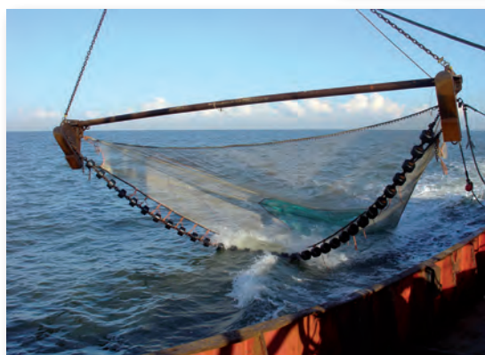
Figure 5: Typical shrimp beam trawl with heavy bobbin rope
